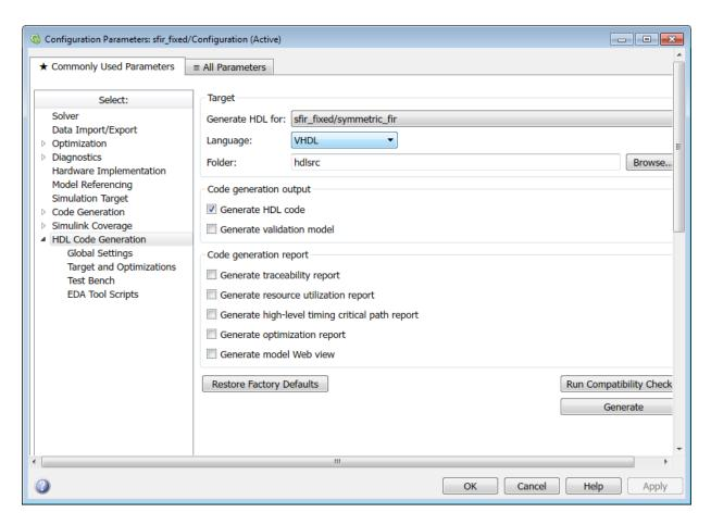
The following figure shows the top-level  $\mbox{HDL Code Generation}$  options pane in the Model Explorer.
